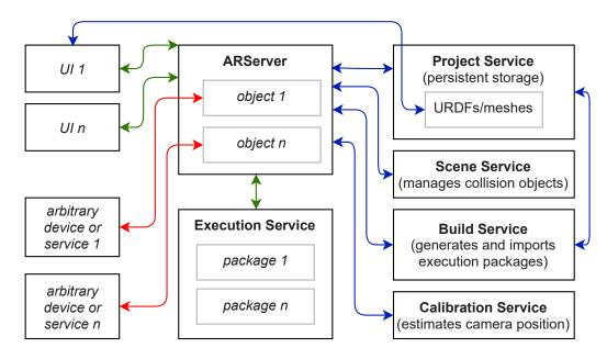
Figure 10.6: Block diagram of the system in a state when object instances are created in the ARServer (scene/project opened and online). Green lines depict WebSockets connections (two-way communication necessary), blue are REST APIs, and for red, an implementer is free to choose appropriate technology.
