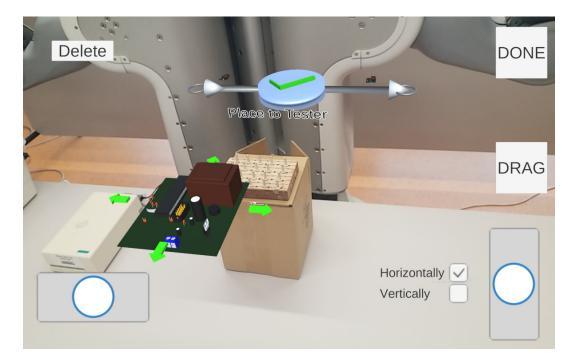
Figure 7.13: Teleoperating user interface for navigating the 3D model of the PCB to the tester device. There are two joysticks on the bottom left and bottom right side of the tablet. Next to the right joystick are two buttons for controlling whether the PCB should move in the horizontal or vertical plane. Above the right joystick is a *DRAG* button. When the user holds it, the 3D model moves in the same direction and speed as the tablet.
