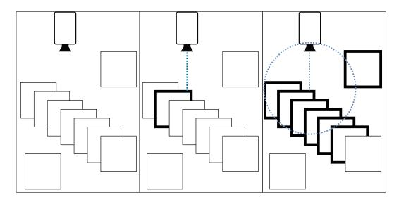
Figure 9.1: Principle of our cluster selection in two dimensions. Left: the camera observes a scene. Middle: a ray is cast from the camera's center and hits an object (square with thick borders). Right: in the position of the hit, a circle (sphere in 3D) is generated and all objects located inside or colliding with are included into the cluster (squares with thick borders).
