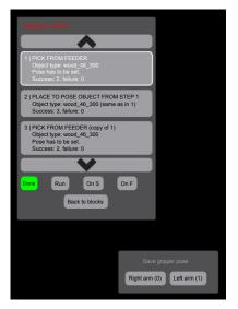
(c) A small dialog shows if the robot is able to detect an object in the feeder and allows the user to save the arm pose.
