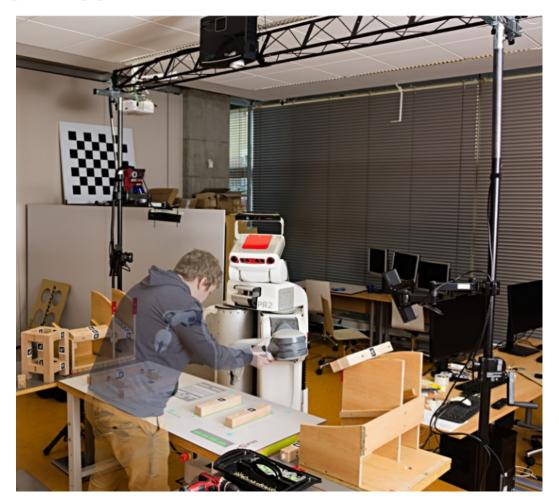
Figure 5.1: Setup of the novel interactive system concept where all the interaction elements (visualization and control) are gathered in a shared workspace (example of setting program parameters using a robotic arm and gestures; image edited).
