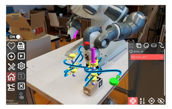
Figure 10.8: The application screen with a tool menu (left), selector menu (right) and noninteractive 3D scene (center), with action points (violet), actions (yellow, green for program loop start, red for its end), logical connections (black/blue) and robot end effectors (magenta). The visualized program realizes a simple pick and place task consisting of low-level actions.
