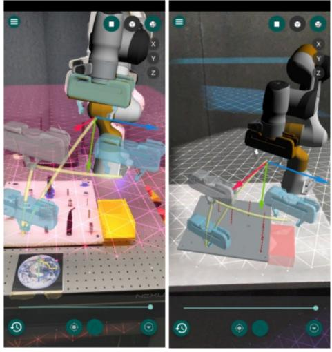
(a) Illustration of the ability to program the (b) Illustration of the ability to program the robot offline directly in the real robot's workspace.
