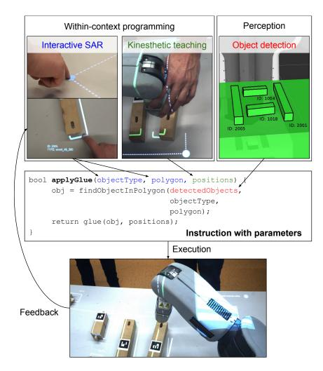
Figure 5.7: Illustration of program parameters' definition (combination of manually set parameters by the user with perceived information by the system) and its execution with visual feedback.
