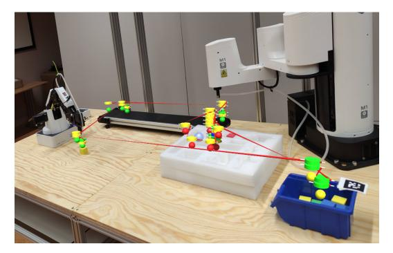
Figure 9.5: The virtual scene rendered over the real environment, used in conducted experiment. The virtual objects represent a simple program, where the small robot should pick a cube, move it to the conveyor belt and pass it to the second robot. The second robot should pick up the cube again, touch the simulated device (represented by a white foam box) in several places with the cube attached, and drop the cube into the blue box.
