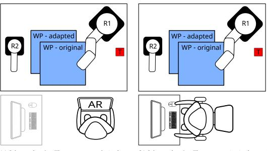
(a) Scheme for C<sub>1</sub>. The person stands in front of the workplace and holds the tablet. The workplace is accessible from the front and the right side. The computer is present but not utilized in this condition.
