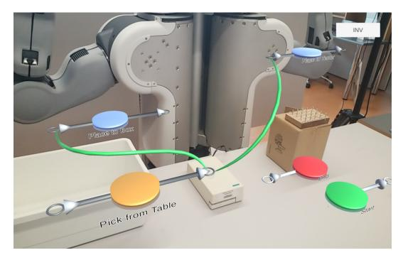
Figure 7.9: Conditional execution of the program. There can be seen *Pick from Table* node, connected with two *Place* nodes. The left and right *nodes* have set different workpieces. The flow of the program is decided during the runtime, based on the workpiece type picked in the *Pick from Table* node.
