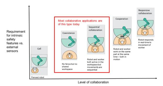
Figure 2.1: Different types of interaction with robots. Reprint from [63].
