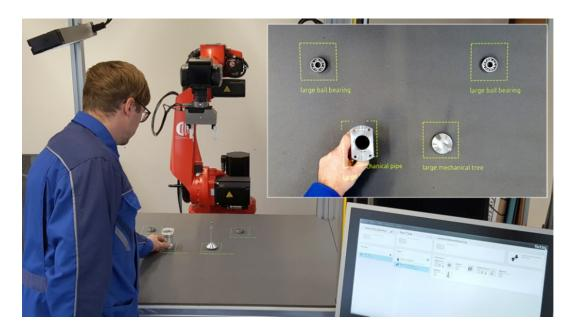
Figure 6.2: Cognitive robotic work cell with features such as object recognition, projectorbased highlighting, hand and body gesture recognition, and touch-based graphical interface for the task-level instruction of the robot. Reprint from [106].
