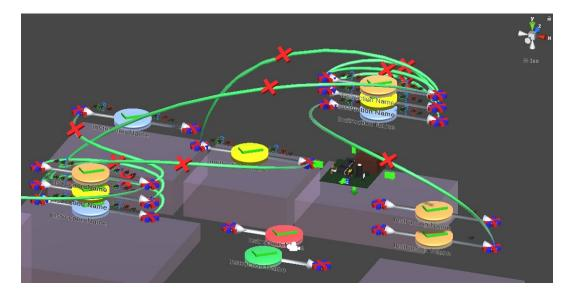
Figure 7.11: Unity scene of the prototype UI. Semitransparent boxes define interactive places, which users can use to define the intended operation. Above each of these boxes, there are *pucks* of various colors, representing different operations. They are connected with green splines, representing the program's flow (for clarity, only a subset of possible connections are displayed in this figure).
