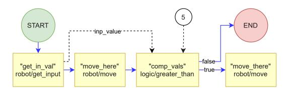
Figure 10.7: The logical structure of an example program. Yellow boxes are Actions (text in quotes is the user-entered name for the instance of Action, below is an object and the corresponding method), blue lines denote logical connections (flow of the program), and black dashed lines denote data connections. The example shows how previous results can be used as parameters of a subsequent action and how logical flow can be branched based on a numerable value (boolean in this case).
