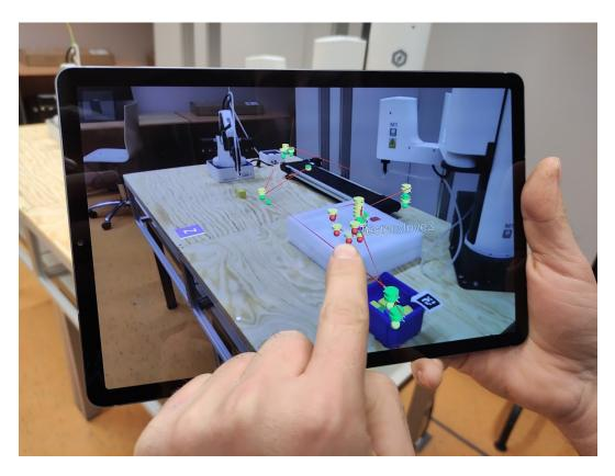
Figure 9.2: Direct touch method. The user selects the object by touching its visual representation on the screen.
