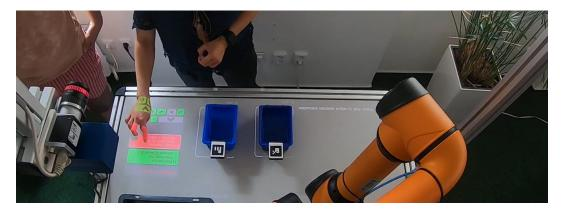
Figure 6.1: Participant programs a visual inspection task using the ARCOR SAR interface.
