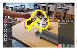
(a) During hand teaching, the robot is locked by the (b) Multiple users collaborating on the task user and therefore unavailable for others, which is indicated within the 3d scene.
