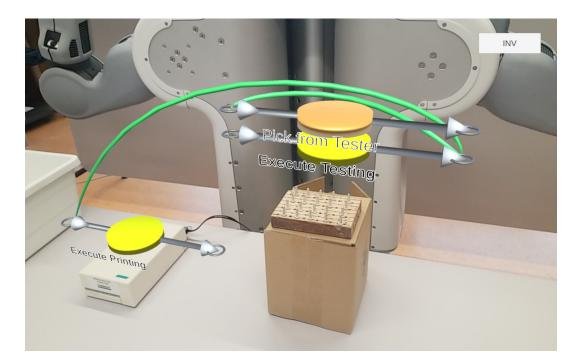
Figure 7.8: Parallel execution of the program. The *Execute testing* node is connected with *Pick from tester* node and *Execute printing* node. All of the *nodes* have set the same workpiece so that both paths will be executed at once during the runtime.
