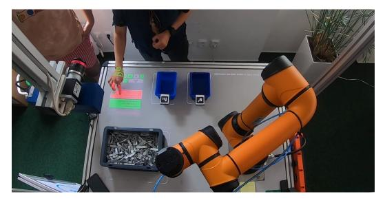
Figure B.2: The projected user interface with integrated robot Aubo i5.
