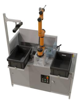
Figure 10.5: Render of a PCB testing workplace with the Ensenso 3D camera for bin-picking, 6 DoF Aubo i5 robot, 2 DoF custom-build robot, functional tester, barcode reader, and printer, source, and target boxes.
