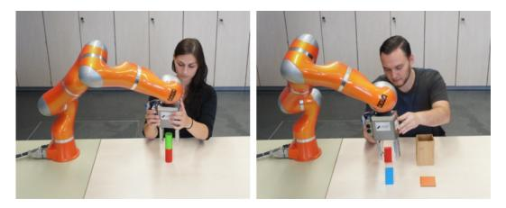
Figure 5.2: User programming the lightweight robot to solve a stacking (left) and sorting scenario (right). Reprint from [101].
