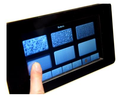
Figure 11.1: The touch screen device is equipped with a haptic feedback<sup>1</sup>. The 2D buttons provide feedback to the user, who can feel the button's texture with the tip of his finger.
