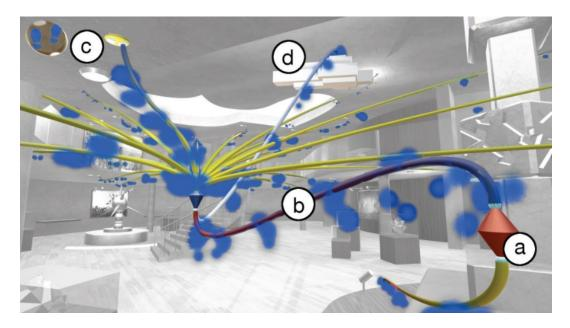
Figure 7.7: Ivy is an immersive visual programming tool for authoring IoT programs and visualizing sensor data. Users can (a) create program constructs, (b) establish logical links, (c) visualize data flows from real-world sensor data and (d) upload data to the cloud. Virtual port nodes (c) act as interfaces to real-world sensors, such as foot traffic readings in this museum scenario. Reprint from [39].
