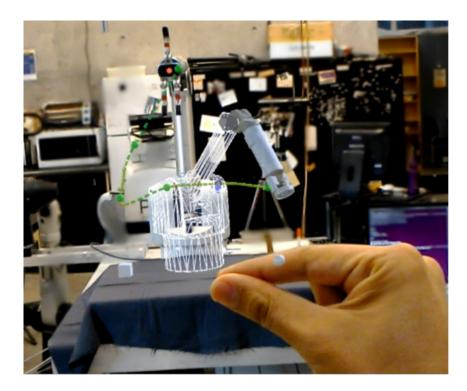
Figure 7.3: A user's point of view from within the Hololens: The user creates, modifies, simulates, and executes a pick-and-place trajectory using our AR robotic system. Notice that the holographic 7-DOF robot arm overlays the real robot and permits the user to simulate motions before execution. All interaction is performed through speech and gestures. Reprint from [111].
