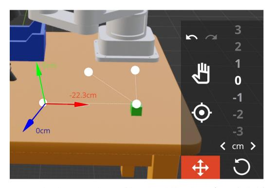
Figure 8.3: The schematic visualization of the tools available in the *transform mode*. The left side contains the 3D widget, so-called gizmo, rendered over the manipulated object. The right side contains the *transform menu*, with several interactive elements.
