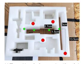
(a) The position of reference points (the red circles) and the trajectory points (the green circles). The first trajectory point's position is referenced with respect to the reference points.
