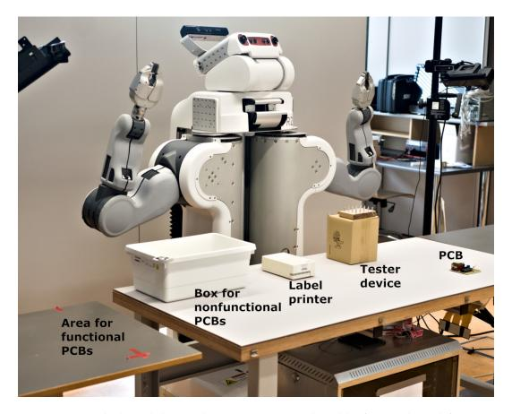
Figure 7.10: Testbed used during the experiment. On the table, from right to left, an example PCB, a mockup of the tester device, a printer of the labels, a box for disposing of nonfunctional PCBs, and another table for functional PCBs.
