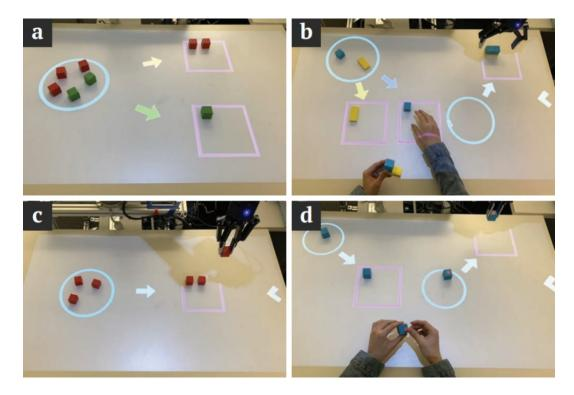
Figure 7.5: Possible applications of PATI include (a) sorting, (b) assembly, (c) alignment, and (d) inspection. The colored arrows in (a) and (b) represent how objects would be sorted based on color attributes. Reprint from [46].
