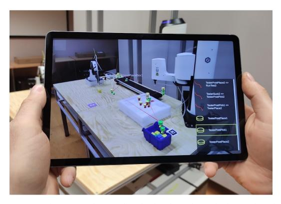
Figure 9.4: Selector menu. The user selects the object by combining the device's physical movement and the object's selection using a side menu.
