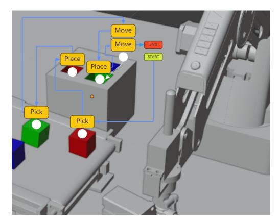
Figure 8.1: The visualization of the SAA concept. The white circles denote the *spatial anchors*, which serve for both the definition and visualization of spatial information. Above each *spatial anchor* is located one or more *actions*, represented by the yellow rectangle. The individual *actions* are connected by the blue lines, defining the program flow. Two *anchors* are connected by the white dotted line representing that the upper *anchor* is positioned relatively to the lower *anchor*.
