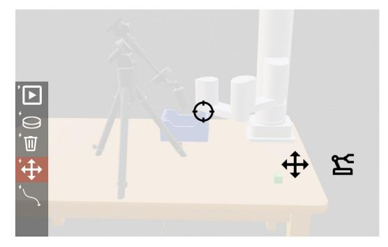
Figure 8.2: Schematic visualization of the user interface. The left side contains the main menu allowing the user to select the appropriate interaction mode. In the middle is a crosshair for indirect virtual object selection. On the right side are two context-aware fixed *mode buttons*, easily reachable by the user's thumb.
