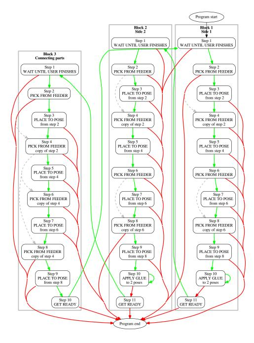
Figure 5.10: Stool production program. The green edges represent *on\_success* transition, while the red ones represent *on\_failure*. The grey edges show dependencies. In the case of *apply glue*, there is a loop. The robot applies glue to one object in a specified area. If an object is found, the program flow continues to the *on\_success* instruction - it tries to apply glue to another object. If there is no object with no glue applied, the flow continues to *on\_failure* (next instruction).
