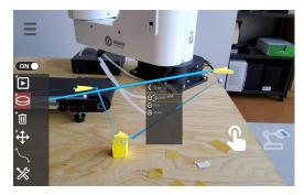
(c) The programming mode. After pressing the mode button, an Action selector menu appears in front of the user, and they can select the Action to be created by selecting it with the crosshair and pressing the mode button.
