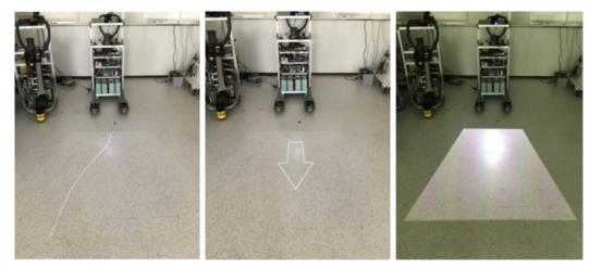
(a) Projection A: trajectory line (b) Projection B: arrow
