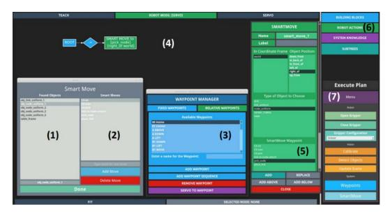
Figure 10.1: Behavior Tree-based user interface. (1,2) Detected objects and associated SmartMoves. (3) Waypoint UI. (4) User's workspace containing the Behavior Tree. (5) SmartMove creation pane; Similar panes allow customization of other operations. (6) List of available operations. (7) Expanded menu containing simple operations the user can perform during plan development. Reprint from [104].
