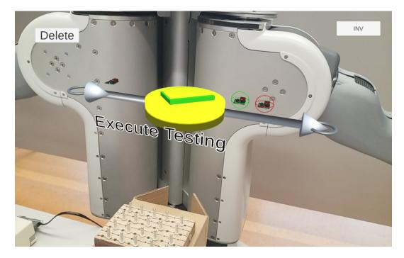
Figure 7.12: The *puck* consists of a central disc, two circles representing the input and the output, and two pipes connecting input/output with the disc. In the prototype, the type of the *puck* is represented by its color and the text placed in front of the disk. Above the pipes, small 3D models of input and output workpieces are placed.
