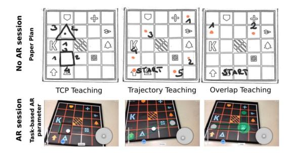
Figure 7.4: Visualization of task-based parameters per task (TCP, trajectory, overlap) in the No AR session (paper plan, top) and AR session (bottom). Reprint from [134].
