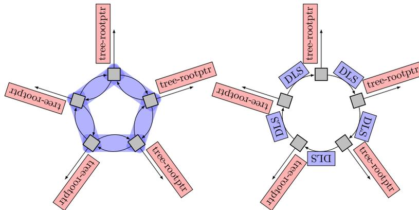
Figure 3.10: On the left-hand side there is the data structure before another folding where the blue areas are going to be folded. On the right-hand side there is the resulting graph with the highlighted parts folded in to the box *DLS*.
