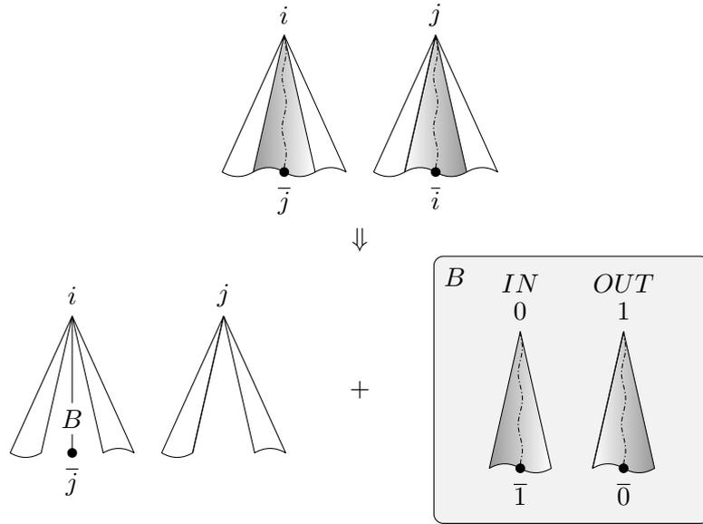
Figure 3.7: An illustration of an elimination of Type 3 cut-points. First, the two components are sliced at their accepting states. Next, the kernels of the result containing references to  $i$  and  $j$  are transformed into a new box  $B$ , which is added to the remaining part of the component  $i$ . Finally, the modified component  $j$  contains no references to  $i$ .
