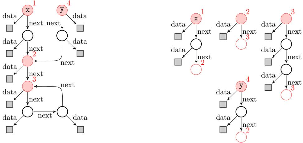
(a) A heap graph with cut-points highlighted in red
