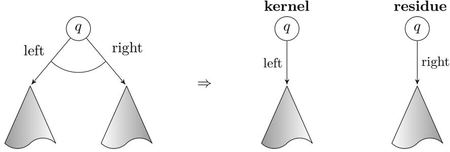
Figure 3.6: An example of component slicing. The left part shows the original automaton that is to be sliced at the state  $q$  according to the edge labeled by “left” (i.e., we perform  $q \rightarrow \langle left, right \rangle (q_1, q_2) \triangleright \{left\}$ ). The right part shows the result after slicing, in which the kernel contains the structure reachable via “left”, and the residue contains the rest of the original automaton (in this case, the structure reachable via “right”).
