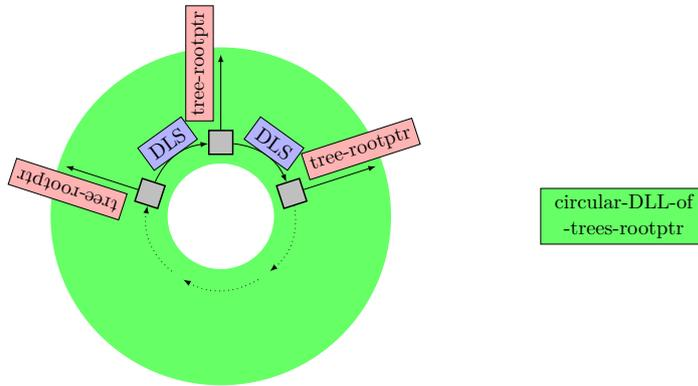
Figure 3.12: On the left-hand side there is the data structure before the last folding. The highlighted green part is going to be folded. On the right-hand side there is the graph with the highlighted part folded to the box *circular-DLL-of-trees-rootptr*. Now, a fixpoint is reached.
