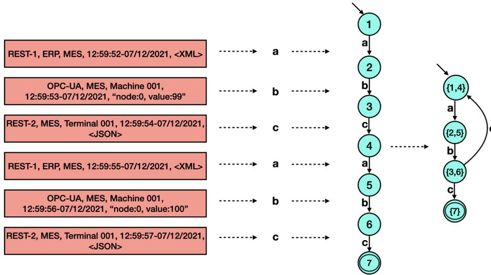
Figure 7.6: Figure illustrates transformation of an event calendar (on the left side) to an automaton. It also contains an automaton created by applying abstraction to the one obtained from the event calendar
