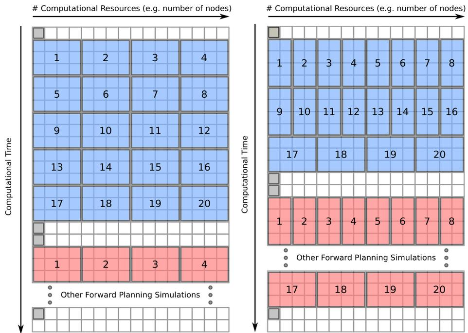
**Fig. 3.** Example of two different execution plans of the neurostimulation workflow on a 16-node cluster. On the left, every job was optimized independently neglecting the queuing times. On the right, the complete workflow was optimized leading to different resources allocations for particular simulations to minimize the overall execution time.
