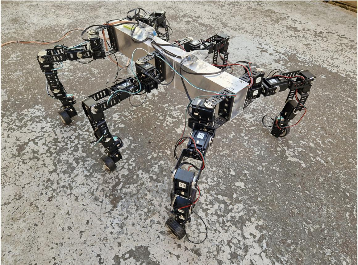
Figure 7.1: WHexaR (Wheeled Hexapod Robot) is a six-legged robot designed and constructed as part of this work.
