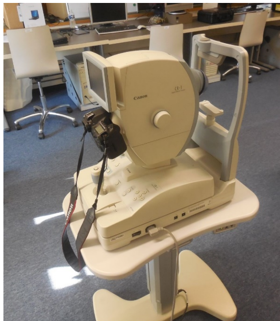
Figure 2.5: Fundus camera Canon CR-1 used in the biometric laboratory at FIT BUT.
