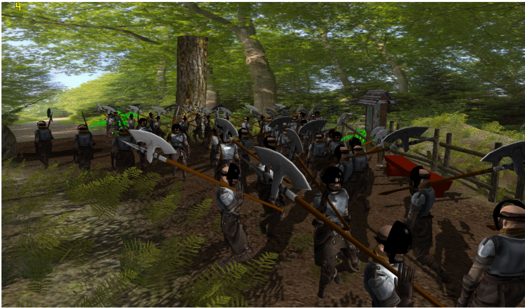
Figure 6.8: Simulated scene with over 40 pedestrians. This scene runs in 4 frames per second, it is mainly caused by the geometry of the character(around 9000 vertices per character, if simulating with more low-poly characters, the performance gets better). Generating images even in this low frame rate is suitable as eventual test data input for people counting or similar systems.
