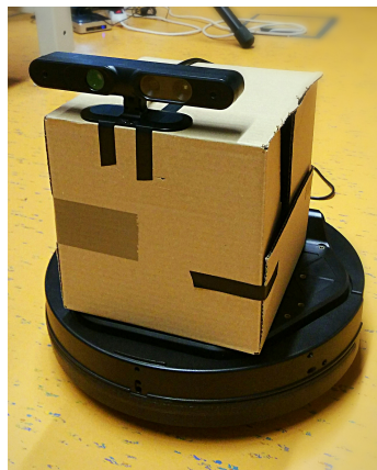
Figure 4.1: My robot for the test purposes, constructed from a kobuki mobile base and an ASUS Xtion depth sensor.
