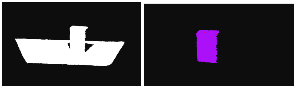
Figure 3.7: Objects detection is done by removing the floor plane points from every received point cloud. Remaining points are points belonging to the detected objects. Segmentation algorithm assigns these points to clusters representing the real detected objects.
