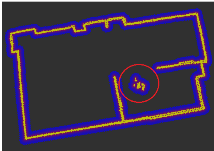
Figure 4.5: An example of a local costmap placed to a global costmap created by the navigation stack.
