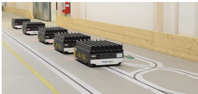
Figure 2.1: Automated Guided Vehicles (AGV) using printed lines on the floor to navigate in indoor scenarios.
