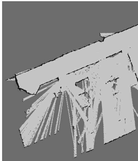
Figure 4.3: The process of building a map using a gmapping package. The black pixels mean the area is occupied, the light gray pixels mean it is a free space, the rest is an unknown area.
