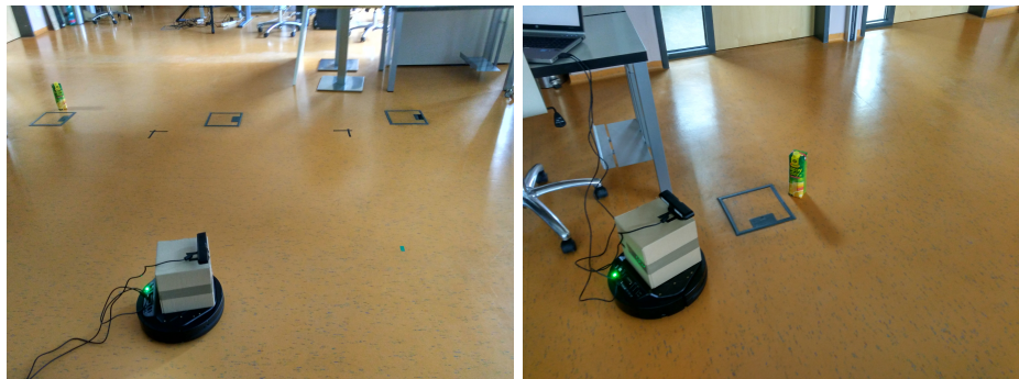
Figure 4.14: The robot accomplishing a goal of finding an object (a juice box in this case).
