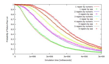
Graph 4.15: Impact of repairing units amount on system with high FU's checkers reliability
