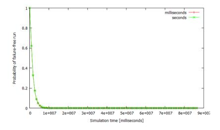
Graph 4.5: Simulations with different time units for numeric method
