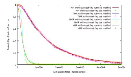
Graph 4.12: Comparism of endurance of systems with growing redundancy
