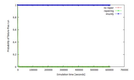
Graph 4.8: Long term simulation with different repairs by numeric method
