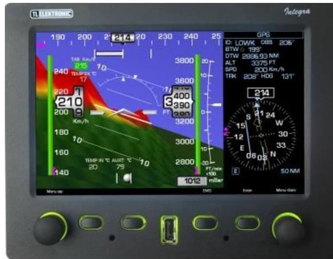
Obr. 15. EFIS&EMS Integra TL-6624 [11]
