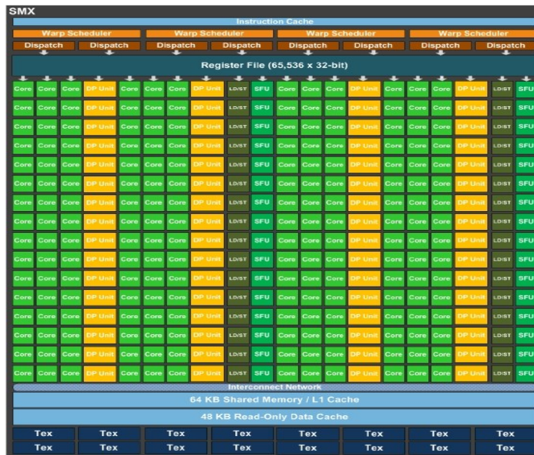
Figure 3 streaming multiprocessor architecture of Kepler class GPUs [10]
