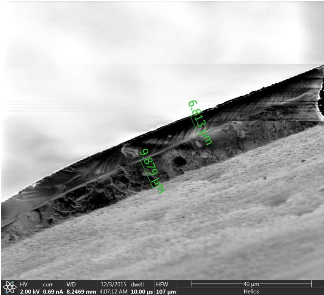
Figure A.8: Layers of CD (coating + ink)
