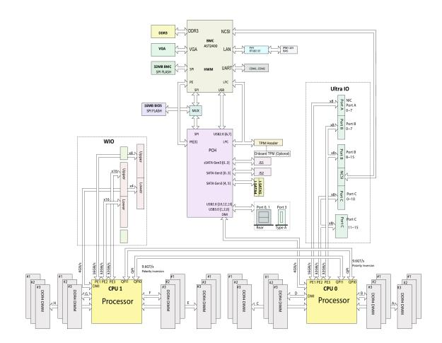
Figure 5.1: Supermicro motherboard's block diagram
