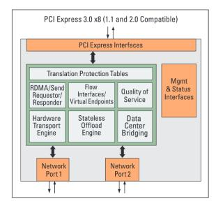
Figure 4.1: Mellanox ConnectX-3 EN block diagram (source: [56])
