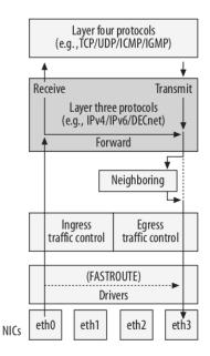
Figure 3.2: Linux kernel traffic flow (source: [45])
