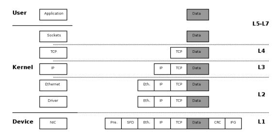
Figure 3.1: Linux kernel layers
