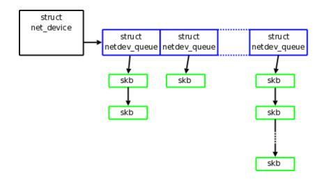
Figure 3.11: Multiqueue device (source: [13])
