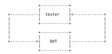
Figure 4.2: RFC2544 test implementation (source: [6])
