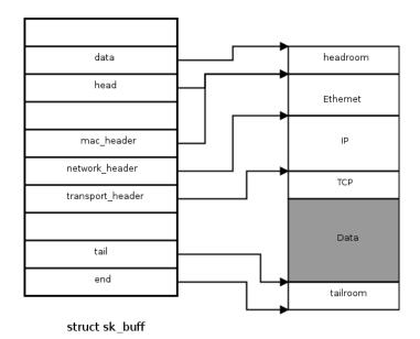
Figure 3.3: Socket buffer structure
