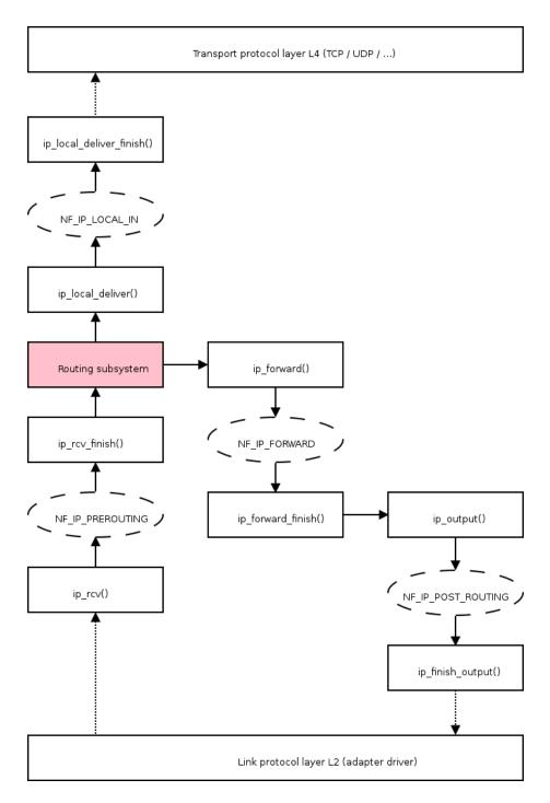
Figure 3.4: Ingress packet processing in the IPv4 stack
