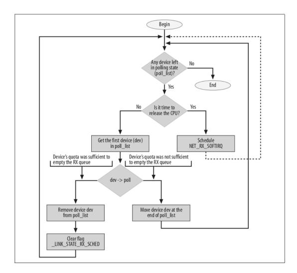
Figure 3.6: Softirq NAPI routine *net\_rx\_action* (source: [5])
