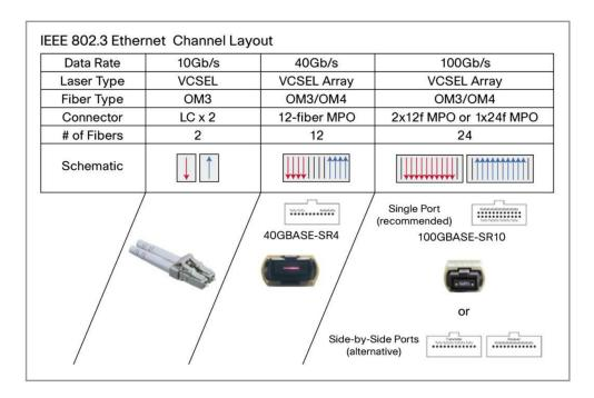
Figure 2.2: IEEE 802.3 Ethernet Channel Layout (source: [8])
