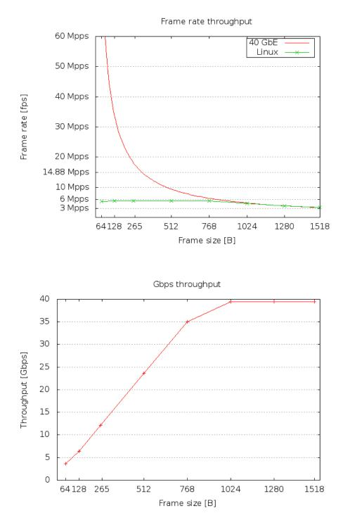
The system is able to perform forwarding at nearly line rate speed with frames 1024 B and larger. The following listing shows the actual interrupt mappings obtained from the /proc/interrupts file.
