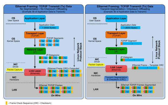
Figure 3.9: Transmit offloads (source: [58])
