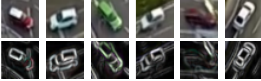
Figure 5.2: Examples of selected target descriptor templates. Each column represents the same target. Upper row: RGB channels of descriptors. Lower row: Edge channels of descriptors visualised in RGB space. Histograms of all descriptors are equalised for a better illustration.
