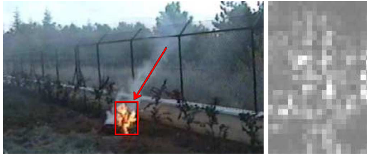
Figure 2.6: Marked fire area and its spatial wavelet transformation's output on the right. Image adapted from article [5].
