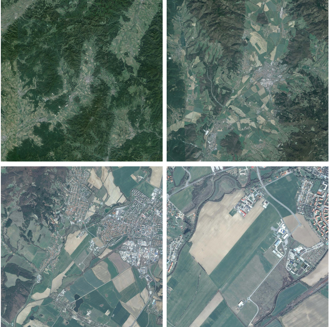
Figure 4.1: Example of 4 textures for various detail levels for area of drop zone Prievidza, Slovakia – each one is 2660 px wide. Exported from Google Earth Pro with camera set at heights 100 km, 30 km, 10 km and 3 km respectively, covering area 63 km, 19 km, 6.3 km and 1.9 km wide.
