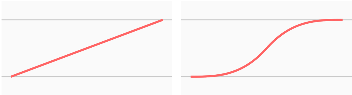
Figure 4.2: Graphs of used TWEEN.js easing functions of time. Left: Linear.None , right: Cubic.InOut
