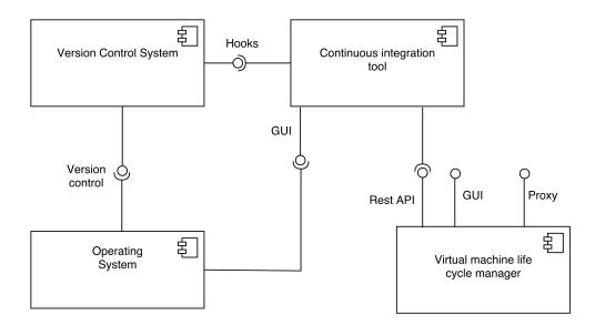
Figure 4.1: System's component diagram.
