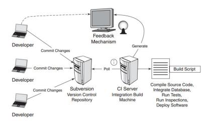
Figure 2.1: Scheme [9] illustrating continuous integration system and workflow.
