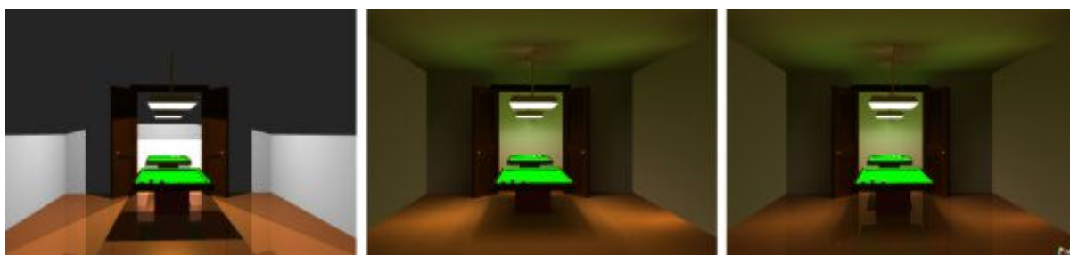
Obr. 2-2: a) ray tracing b) radiozita c) kombinace ray tracingu a radiozity
