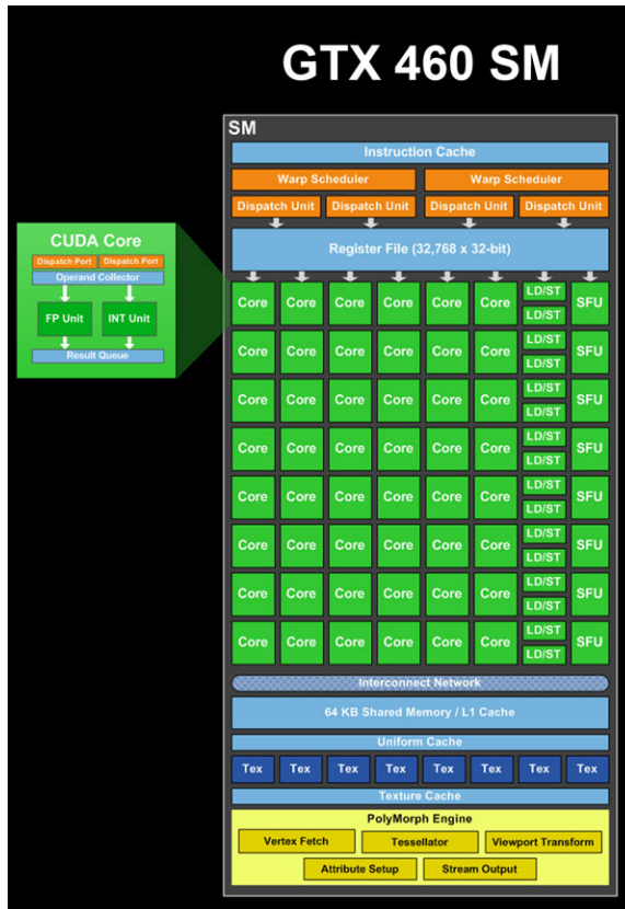
Figure 4.1: Architecture of a stream multiprocessor of GTX460 graphic adapter.
