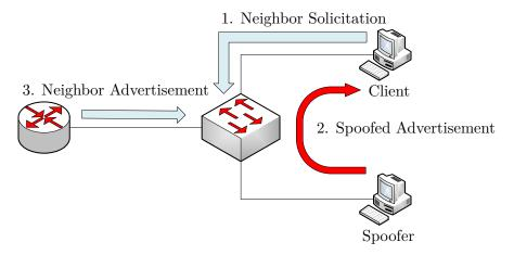
Figure 4.5: Schema of IPv6 Neighbor Spoofing
