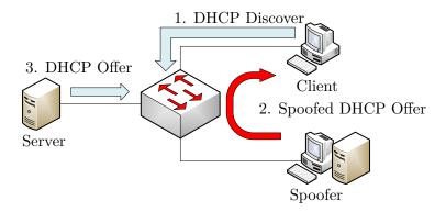
Figure 4.1: Schema of DHCP Spoofing
