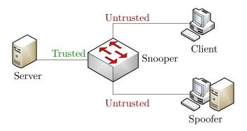
Figure 4.3: Schema of DHCP Snooping
