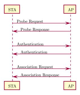
Figure 3.1: Sequence of WEP Open System Authentication
