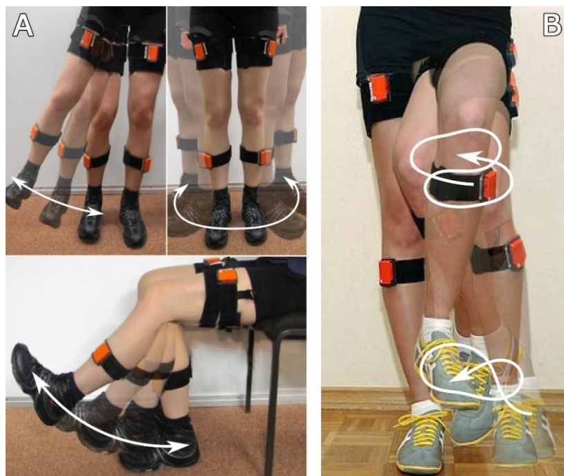
Figure 3.6 calibration procedure using predefined (A) vs arbitrary (B) movements [18]
