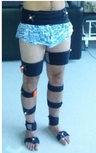
Figure 5.5 Optitrack reflective markers placement
