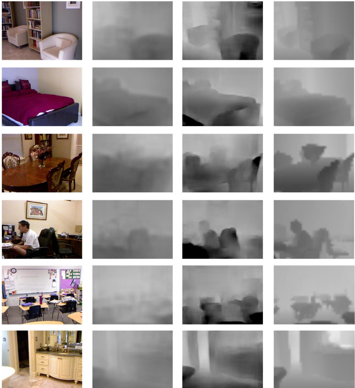
Figure 5.8: From left to right: input image, produced by model by Eigen et al. [5], output of the proposed model, the ground truth
