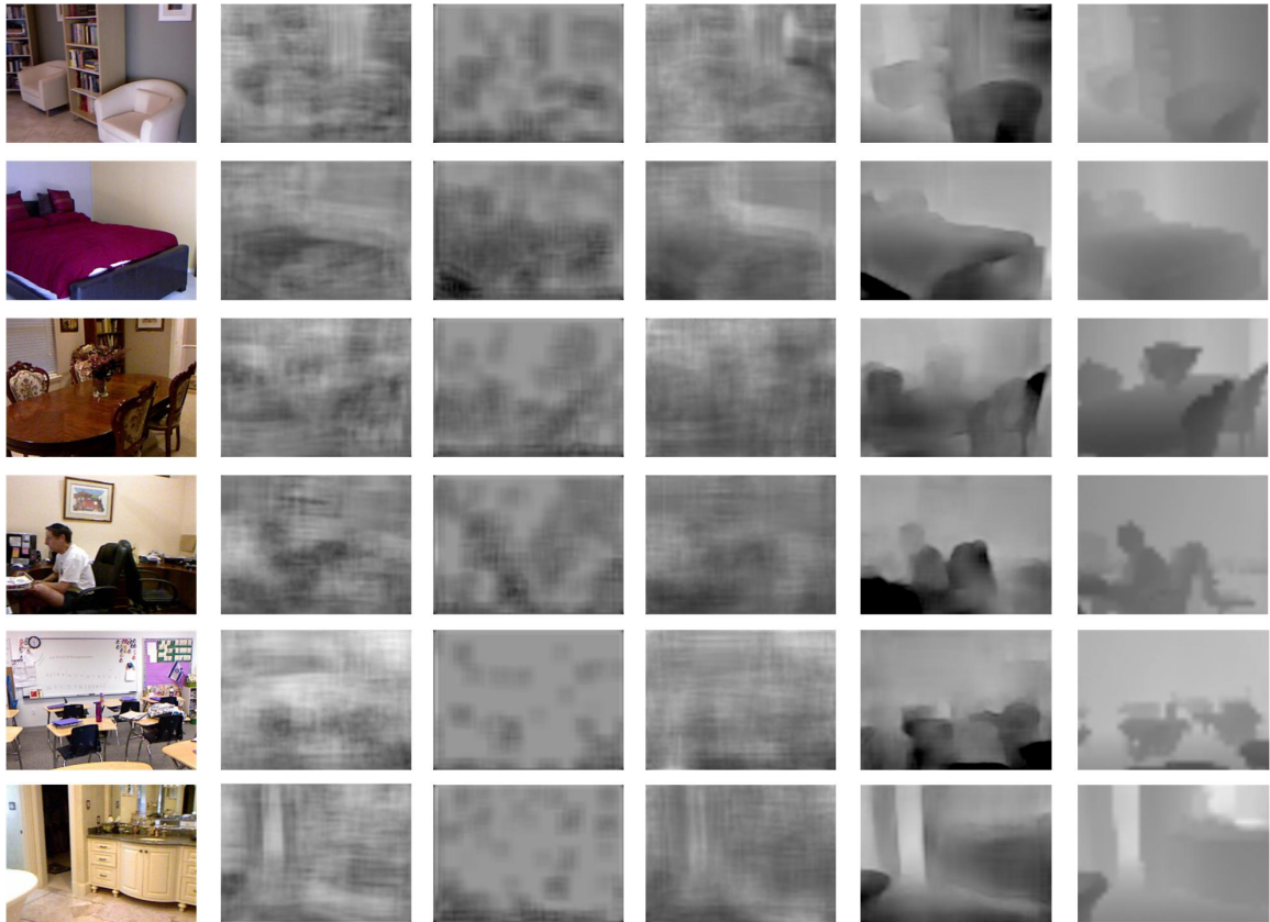
Figure 5.6: Qualitative comparison of the outputs of the refining network trained with different loss functions. From left to right: input image, output of the network trained using abs loss, abs log loss, sc-inv + abs loss, norm. + abs loss, the ground truth
