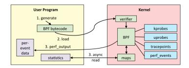
**Figure 2.5:** The eBPF workflow which consists of generating the BPF bytecode, verifying it, running it via the virtual machine (engine) within the kernel and storing the resulting raw data into the BPF maps or directly as a **perf** output. The illustration is taken from [25].
