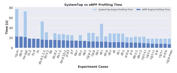
Figure 8.4: Comparison of the SystemTap and eBPF engine, featuring all of the methods and pipelines, and a selected subset of the total experiment cases. Specifically, we kept only the first iteration of every case since the values of subsequent iterations were rather similar.
