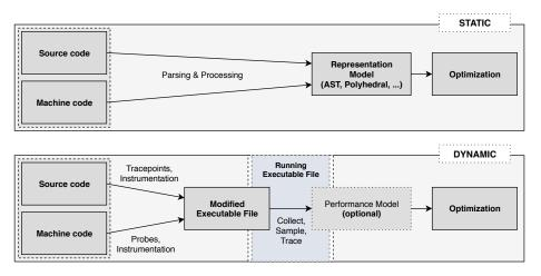
**Figure 2.1:** An illustration of the different analyses in the field of performance analysis. Both static and dynamic analyses usually leverage source and machine code to either parse and process or inject instrumentation, respectively. The biggest difference is that dynamic performance analysis needs to run the executable file in order to obtain performance data.
