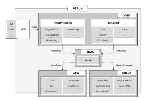
**Figure 4.3:** A simplified architecture schema of the Perun featuring four main components (*logic, data, view* and *check*) as well as the VCS module: interface to Git, SVN and similar systems. The Data layer is a core component that handles operations related to the generation and manipulation of profiles. The profiles are further used by the postprocess, view and check components to analyze, visualize or compare the raw performance data.
