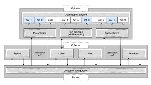
**Figure 6.3:** A schematic module overview of the new optimization layer and its interaction with the **runner** and collectors. The **runner** has been modified to automatically perform the optimizations (if enabled) between the selected collection phases, independently of the specific collector. Blue modules represent selected optimizations for some concrete run.
