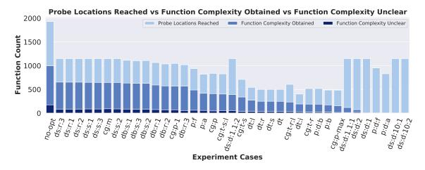
**Figure 8.3:** Numbers of function performance models that we can infer from data collected by each case with (1)  $R^2 \ge 0.5$  (Function Complexity Obtained), or (2)  $R^2 < 0.5$  (Function Complexity Unclear). Functions with less than three records were omitted.
