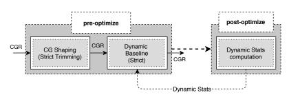
Figure 7.5: A schematic overview of the *Basic* pipeline that utilizes the Call Graph Shaping (in strict trimming mode) and Dynamic Baseline (in strict mode). The methods leverage both the Call Graph Resource (CGR) and Dynamic Stats, however, since the Dynamic Stats are computed after the profiling, it can be utilized only in the next profiling.
