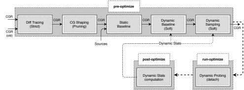
Figure 7.7: A schematic of the Full pipeline. Compared to the previous pipelines, the Full pipeline also utilizes the *run-optimize* phase by including the Dynamic Probing.
