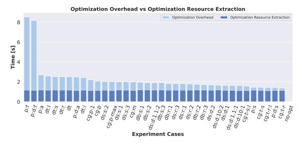
Figure C.3: A complementary Figure to the Figure C.2 that shows the same OO and ORE metrics, however, measured with the *cache\_on* configuration. Note especially the significant reduction of ORE values.
