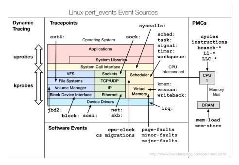
Figure 2.4: A scheme of the available perf events, their categories (such as *dynamic tracing, static tracing, hardware and software events*) and the corresponding tracing and sampling mechanisms (*kprobes, uprobes, tracepoints, performance monitoring counters*, etc.) arranged into a map. The map illustrates the essential system components, e.g. file system, virtual memory, networking, drivers, scheduler, communication buses, etc. Taken from [26].
