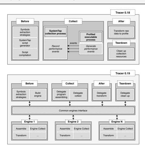
Figure 6.1: A schematic overview of (a) the old Tracer architecture (v0.18) with hardcoded SystemTap usage, and (b) the proposed architecture (expected as version 0.19) that abstracts away supported instrumentation frameworks. The collection process itself is divided into four separate stages: before, collect, after and teardown. Each light grey box represents an action, while the arrows represent callback of functions.
