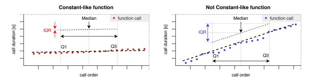
Figure 7.1: A comparison of constant (red) and non-constant (blue) behaviour. The idea is to compare the IQR (*interquartile range*) and *median* values of the function's data set: when the IQR/median ratio is sufficiently small, we assume that the function is constant.
