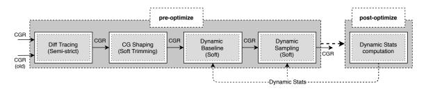
Figure 7.6: A schematic illustration of the Advanced pipeline. Compared to the Basic pipeline, both the Dynamic Baseline and Dynamic Sampling methods trigger the Dynamic Stats computation in the *post-optimize* phase. Moreover, apart from the CGR, the Diff Tracing method also leverages the CGR of the previously profiled project version.
