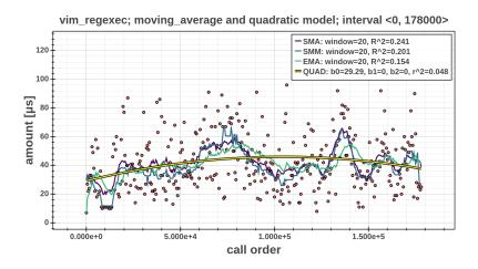
**Figure 3.3:** An example of moving average variants (*simple moving average* (SMA), *simple moving median* (SMM) and the exponential moving average (EMA)), and the regression analysis quadratic model (QUAD). The x (resp. y) axis represents the call order of the function vim\_regexec (resp. function runtime). Taken from [66].
