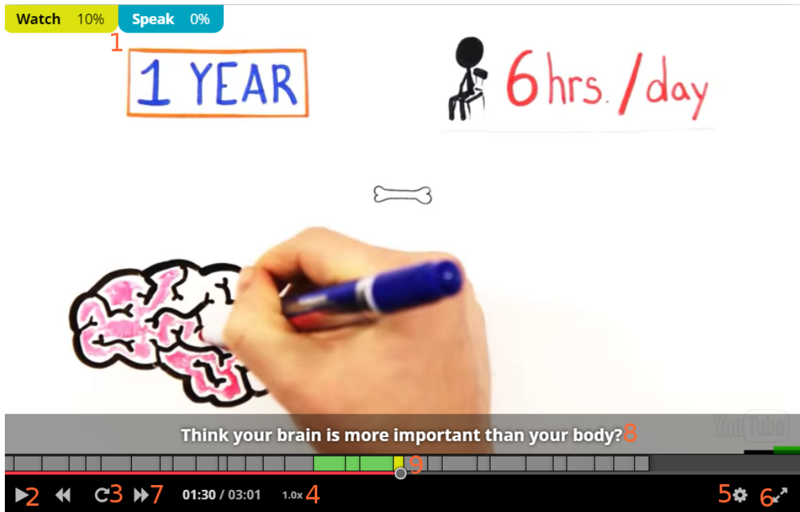
Figure 4.2: GPlayer version 0.8. On the top left corner there are modes we can play the video in. 'Play/pause' button is on the bottom left corner. Next to play button is 'Play previous segment' button that is available only in watch mode. Next on the right is 'Repeat segment' button, followed by 'Play next segment' button that is available only in watch mode, then time played and total time of the video are displayed, then 'Speed customization button'. On the bottom right are two buttons: 'Change settings' button and 'Full-screen' button. Above this bar is a segments section, every segment is clickable. On the top of segments section are subtitles for currently played segment.
