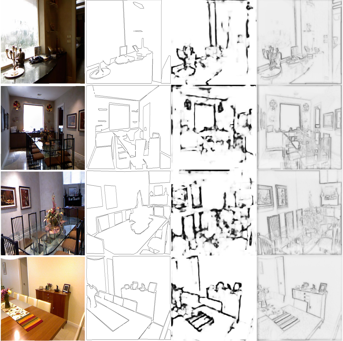
Figure 7.5: Results over the NYU depth V2 dataset. From left original image, ground truth, Own RCF based model, Own RCN based model.
