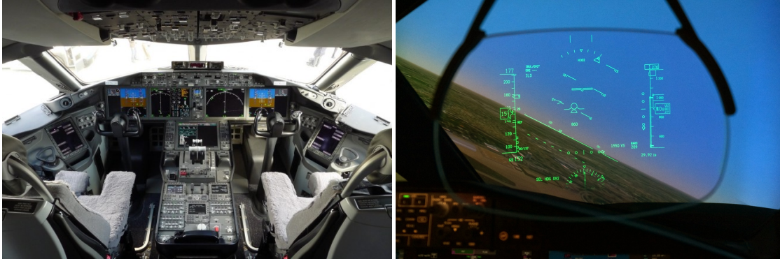
Figure 4.1: Boeing 787 cockpit and HUD [20] [17].
