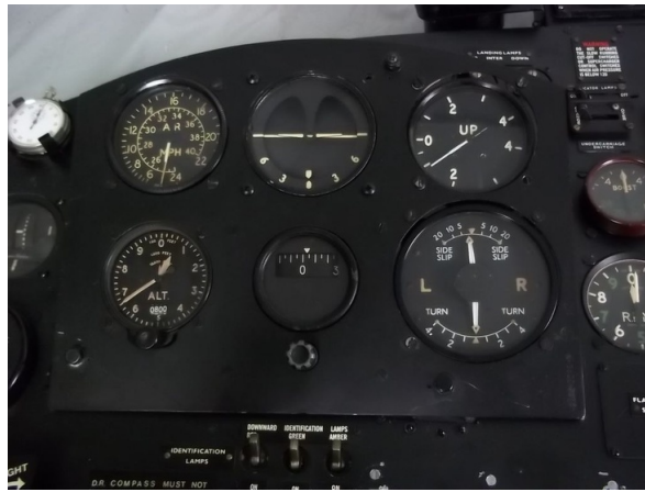
Figure 3.1: Avro Lancaster basic six layout [21].
