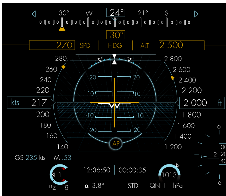
Figure 6.13: Display with Flight Director and Autopilot.
