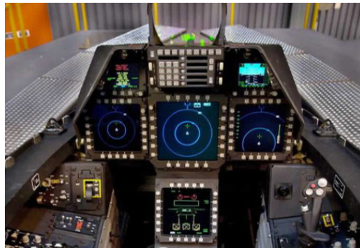
Figure 4.4: Locked Marting F-22 Raptor cockpit (instrument panel)[16].
