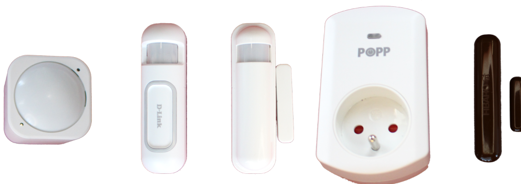
Obr. A.4: Z-Wave zariadenia – Aeotec Multisenzor 6, Dlink DCH-Z120, Philio PST02-1C, Popp 123627, Fibaro FGK-107
