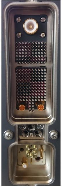
Fig. 3.1: ARINC 600 connector on LRU backplane
