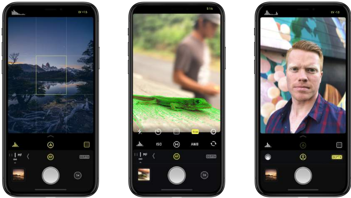
Figure 2.5: Halide application screenshots from Halide’s Press Kit [3]. The leftmost picture shows a screen of Halide’s user interface. The camera view-finder contains the adaptive level grid. In the top left corner, a live histogram indicates the current exposure. In the right corner, the application shows the current exposure value. The second screenshot from the applications displays the focus peaking feature. The last screenshot shows the portrait view while taking a photo from the front camera.
