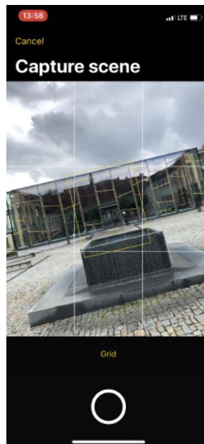
Figure 4.8: Screenshot from the application showing a camera screen with a grid and a rectangle representing the device's alignment level. The rectangle helps the user align the device with the static grid.
