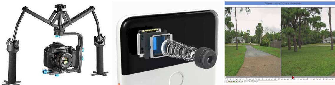
Figure 1.1: 3 approaches in video stabilization
