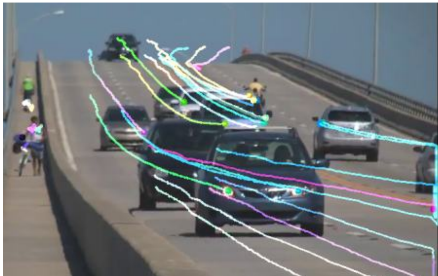
Figure 2.3: Cars tracking using optical flow by Lucas Kanade algorithm 2
