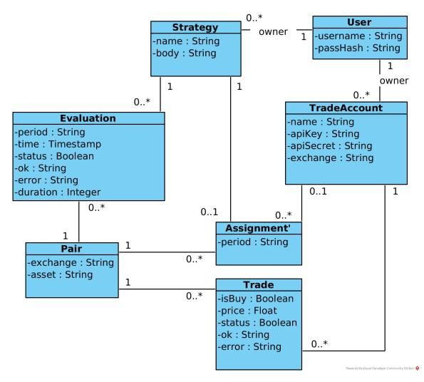
Figure 4.4: Entity-Relationship diagram of system data
