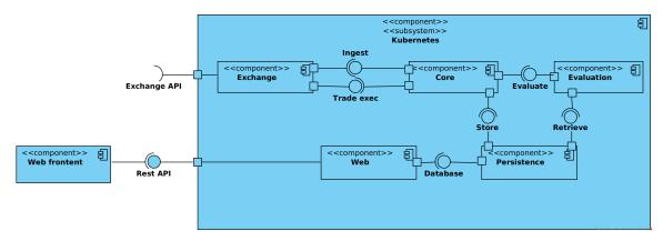
Figure 4.1: Component diagram of basic architecture
