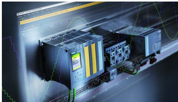
Obr. 2.1: Moderné PLC Siemens Simatic S7-1500
