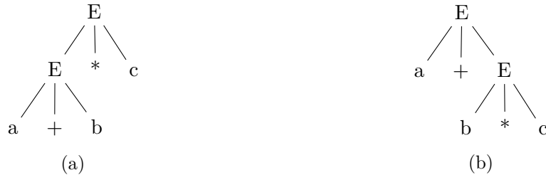
Figure 1.1: Parse trees of a + b * c produced by G in example 1.13 using leftmost derivations
