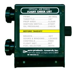
Figure 3.9: C-46 Commando aircraft scroll checklist<sup>11</sup>.
