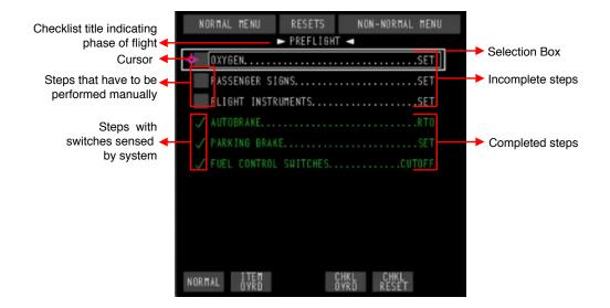
Figure 4.4: Pre-flight checklist related to normal procedures $^{6}$ .
