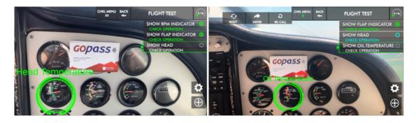
Figure 6.11: Left: Flight instrument marking in the default mode. Right: An active step can be deferred through Defer button.
