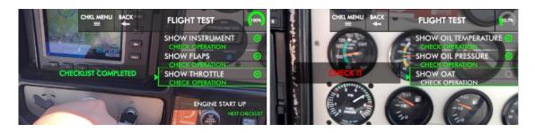
Figure 6.13: Left: Message indicating completion of the checklist. Right: Active task was confirmed but flight instrument was not even in the field of view.
