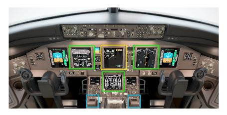
Figure 4.2: Boeing 777 flight deck layout<sup>4</sup>.
