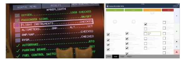
Figure 3.11: Left: Boeing 777 electronic checklist<sup>13</sup>. Right: Application on iPad<sup>14</sup>.
