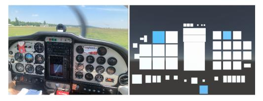
Figure 7.2: Comparison of flight deck on the left side and virtual 3D model on the right side. Model elements marked blue represents an image markers.
