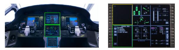
Figure 4.7: Left: PC-12 cockpit flight deck<sup>9</sup>. Right: System MFD display layout<sup>10</sup>.
