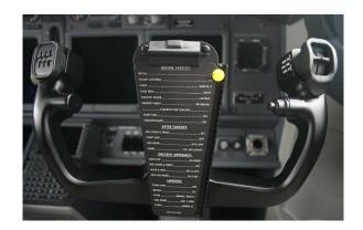
Figure 3.8: Checklist attached to yoke in Boeing  $737^{10}$ .
