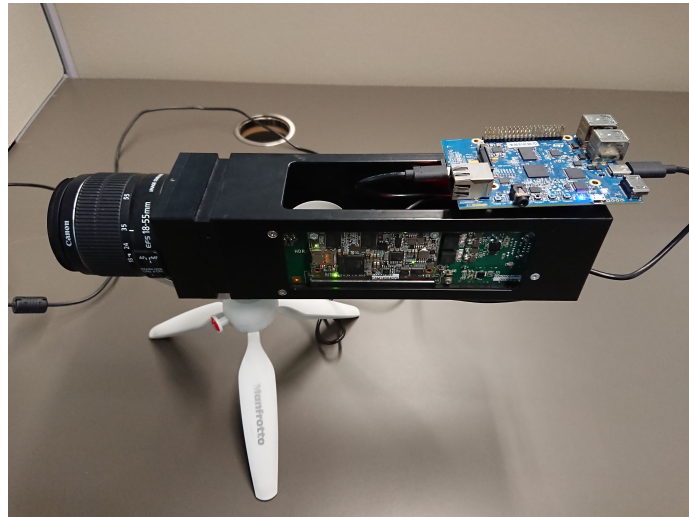
Figure 5.2: Intelligent camera sensor connected to the STM32MP1.
