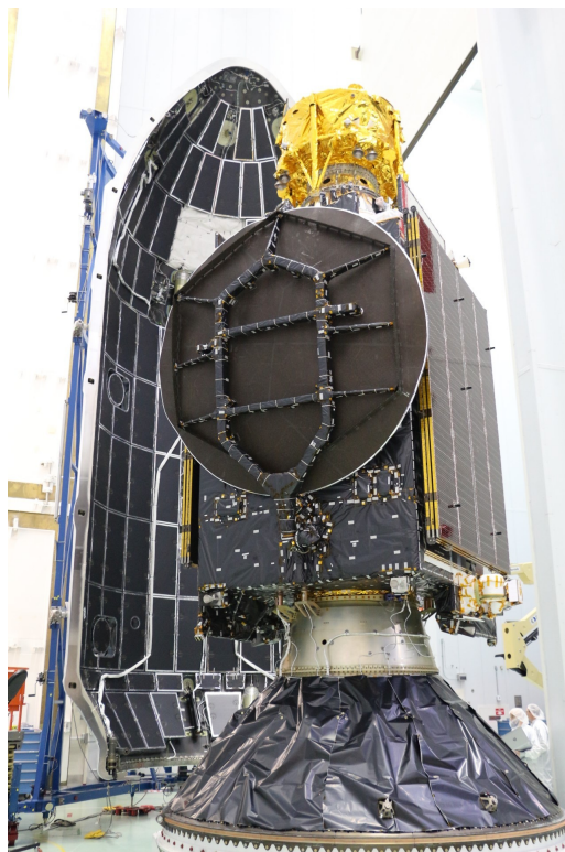
Figure 2.1: The Beresheet spacecraft and the Nusantara Satu launch configuration with a 13.1 meters tall Falcon 9 payload fairing in the background. Taken from [23].
