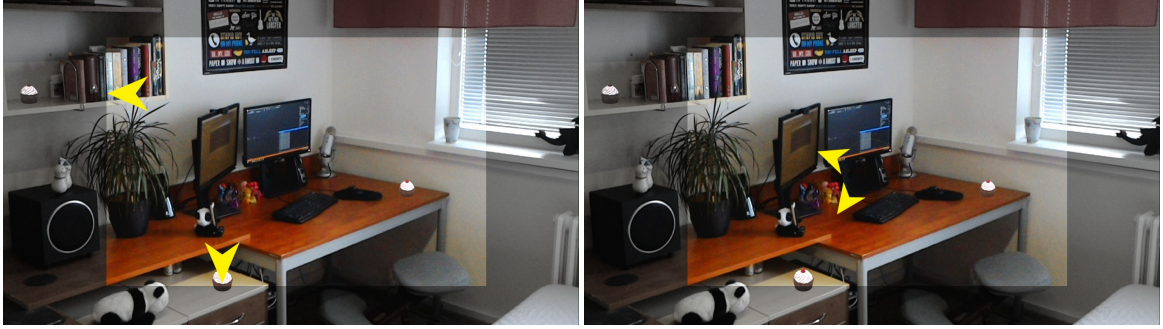
Figure 4.3: Two possible cursor designs. Border (left) and center circle (right) directional indicator. Picture differs display part where holograms are visible from non-hologram-visible part
