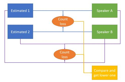
Figure 4.1: Permutation invariant training procedure.
