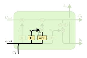
Figure 3.6: Input gate layer[13].
