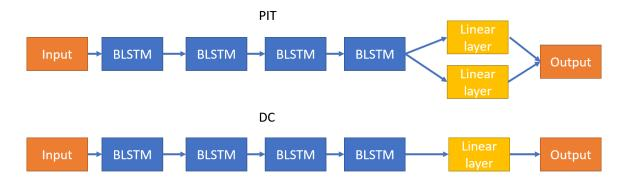
Figure 6.3: The NN architecture for training with PIT and DC method.
