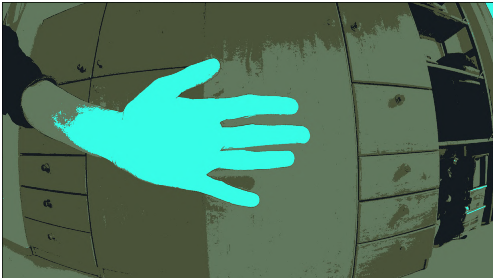
Obr. 3.4: Zhlukovanie pomocou K-means N = 4 .
