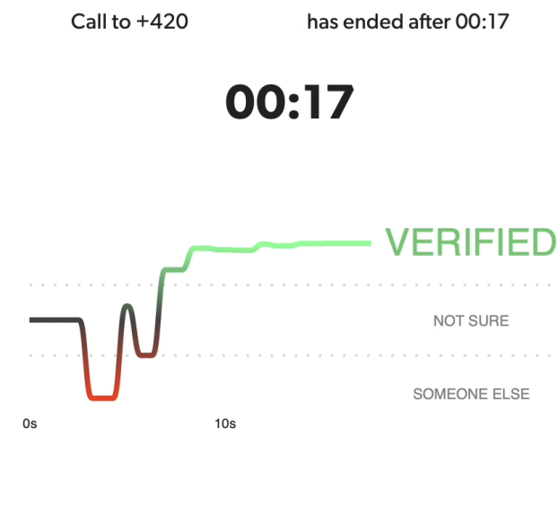
Figure 6.2: Screenshot of complete verification graph of deepfake recording created using Overdub feature of Descript. A big drop is visible right at the beginning, afterwards the course reproduces the genuine verification graph.
