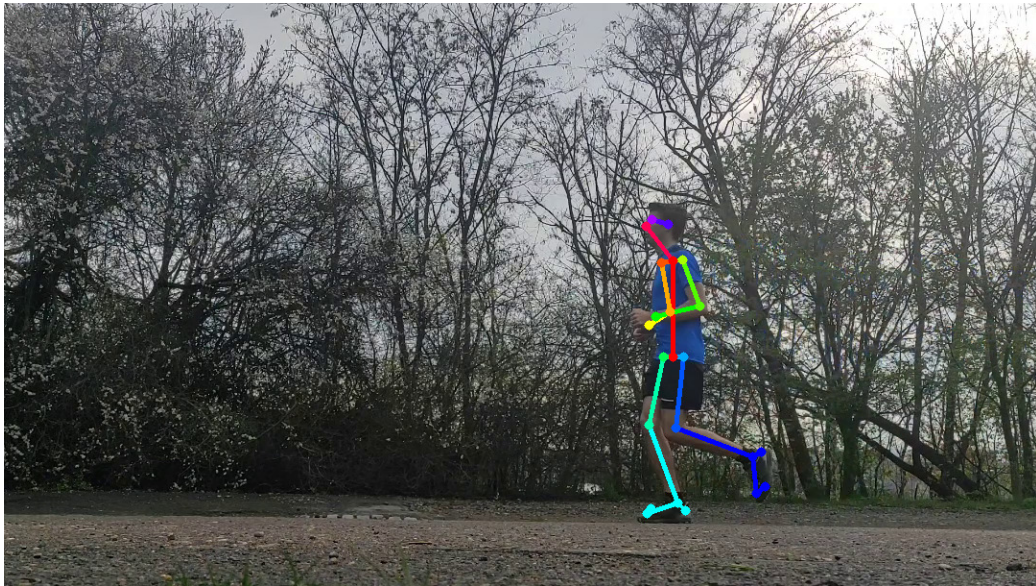
Figure 5.15: One frame during the stance phase. The runner has limited knee flexion at this moment, which might indicate excessive strain to the knees during running.
