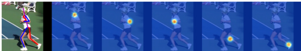
Figure 3.7: Example of the heatmap application for joint estimation [4]
