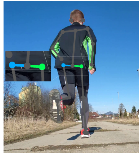
Figure 4.7: LHip and RHip key-points used for pelvic drop analysis from a posterior recording.
