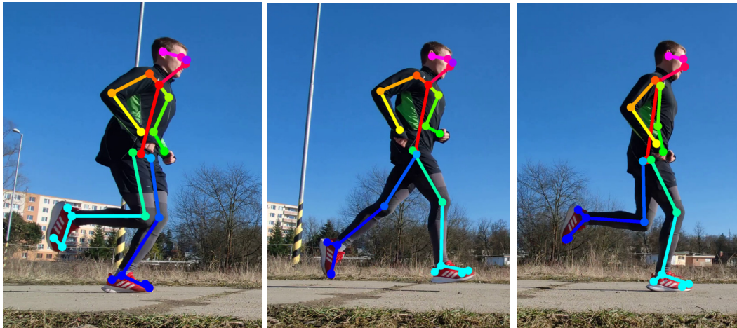
Figure 4.5: Three frames with horizontal foot detected. The second one is mid-flight and needs to be filtered out.
