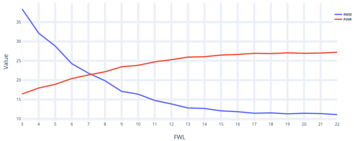
Figure 6.11: Results of using 32-bit arithmetic with different FWL and IWL settings.
