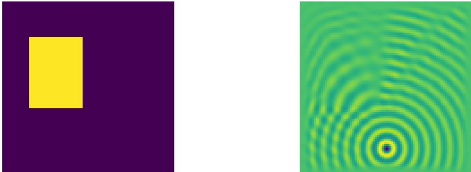
Figure 3.2: Figure shows the sound speed distribution of the domain with a size of 96x96. However, instead of an idealized skull model generated as a sum of several circular harmonics, this sample contains a filled rectangle and its predicted wavefield using a neural network. The \ell_\infty error after 1000 iterations is below 0.45%. This sample's inference (1000 iterations) took 4.54s using 1 GPU on the Karolina supercomputer.
