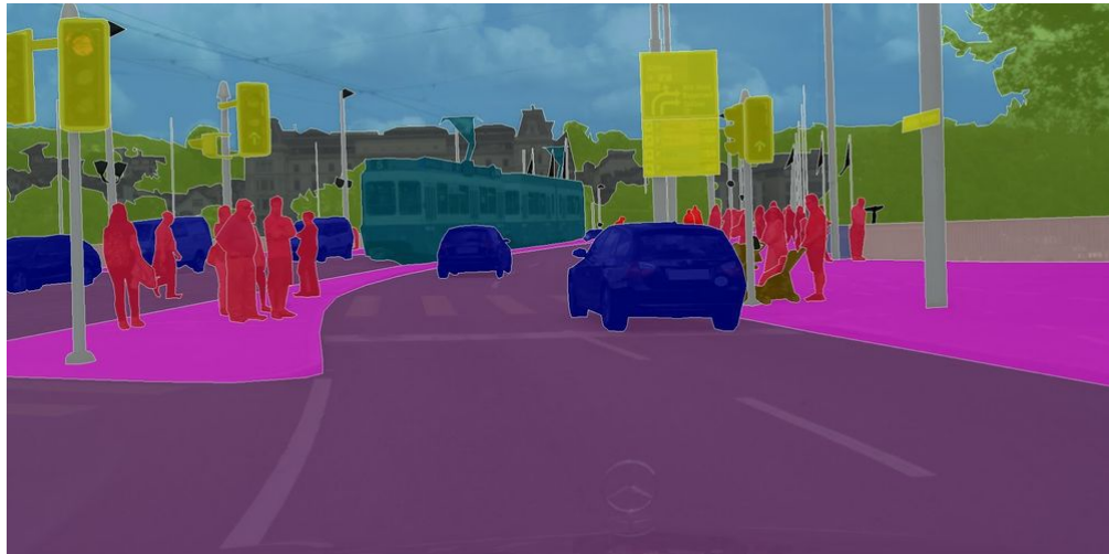
Figure 2.4: Objects from the same class are masked with the same color. For example, vehicles on the road are blue, nature is green, buildings are gray, the road is purple, etc... This image can serve as an example of an autonomous system – a self-driving car. The image was taken from [16].
