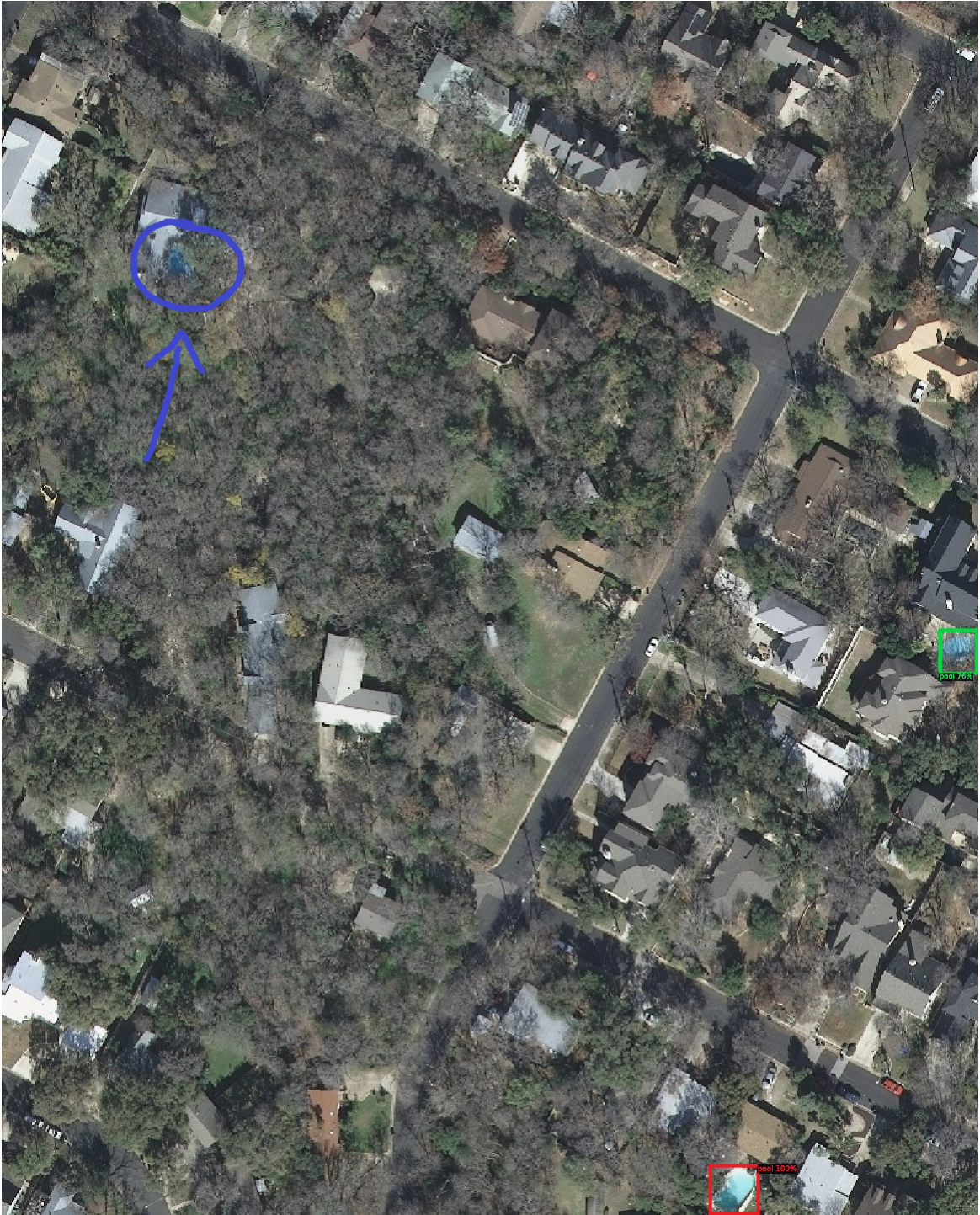
Figure 6.2: The blue circle in the upper left corner of the image indicates the missed detection. This pool is covered by trees and is really difficult to see it even by a human.
