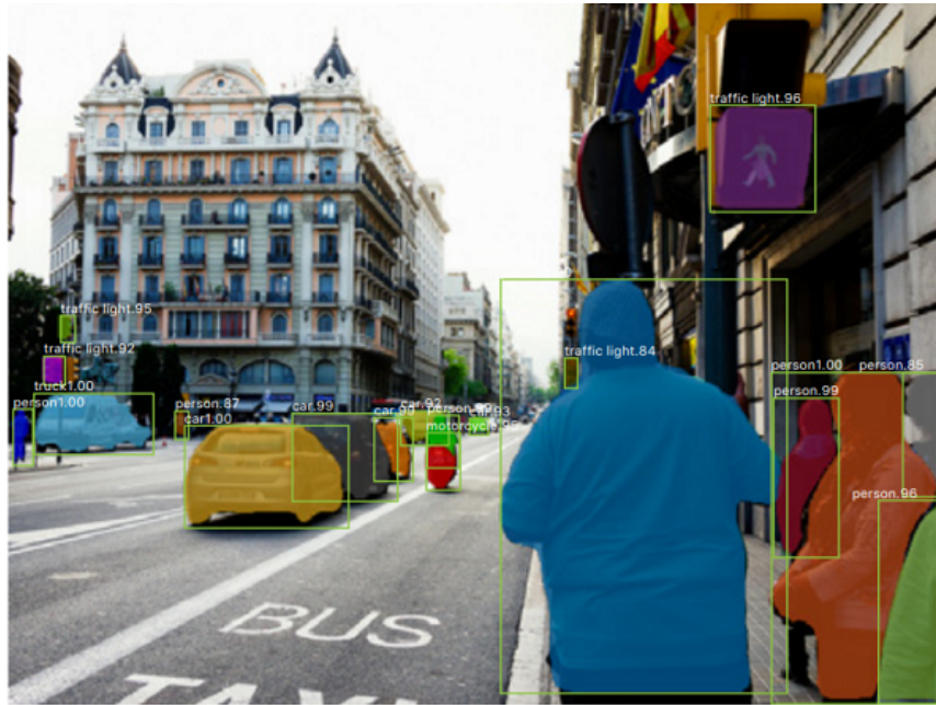
Figure 2.6: The example of instance segmentation using the Mask R-CNN deep learning model. As it can be seen, it is a combination of object detection (bounding boxes around the objects) and semantic segmentation. The image was taken from [13].
