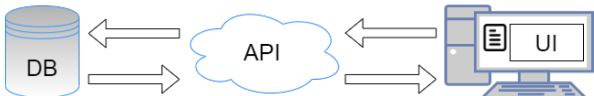
Figure 5.3: The tool consists of three parts that communicate with each other by sending requests.
