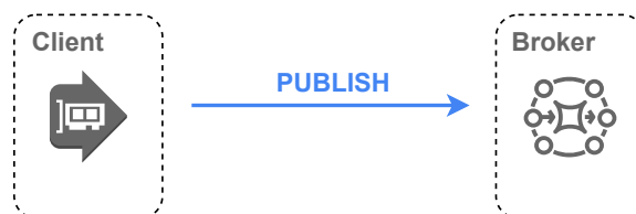
Figure 3.2: Quality of Service level 0 schematics
