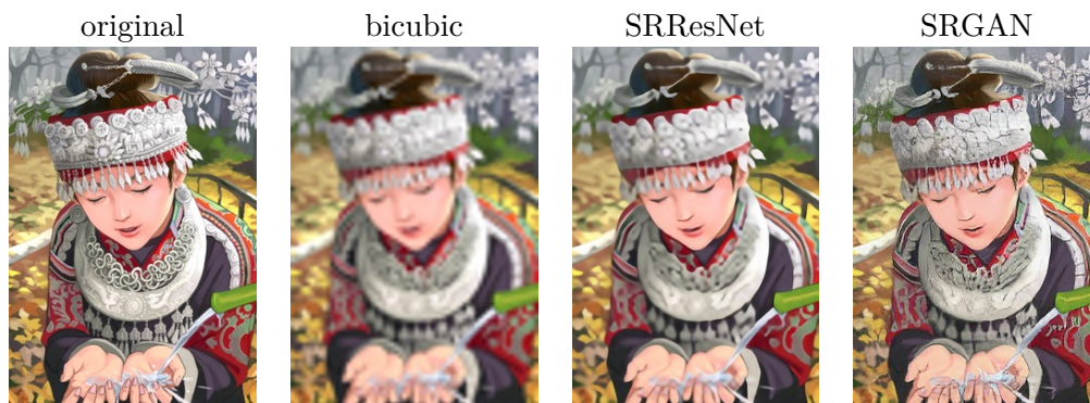
Figure 4.12: The preview of original and super-resolution obtained images from various techniques. The significantly better visual quality performed the SRGAN model. Adapted from [25].
