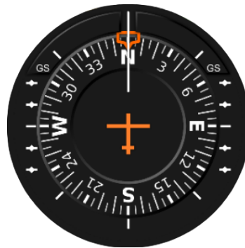
Figure 2.5: Heading Indicator with a heading bug set onto the North.
