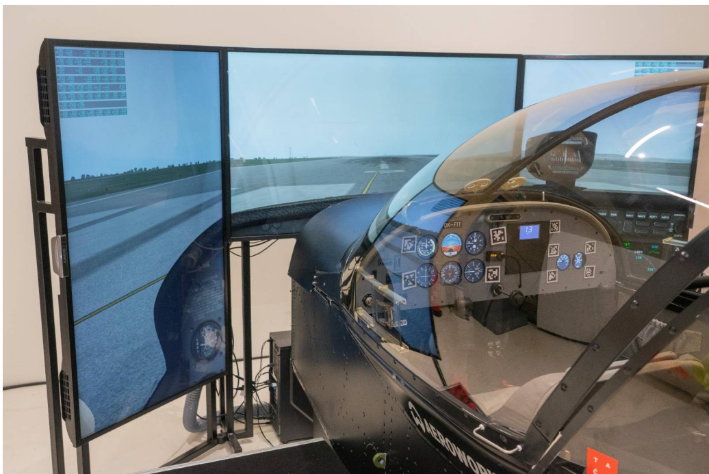
Figure D.1: Visualization subsystem of the SimStar simulation framework.
