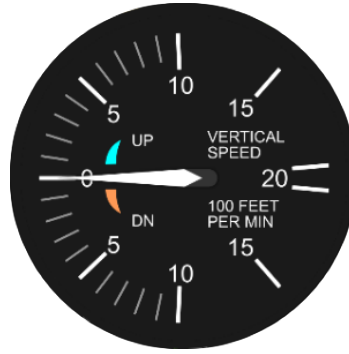
Figure 2.4: Vertical Speed Indicator gauge.
