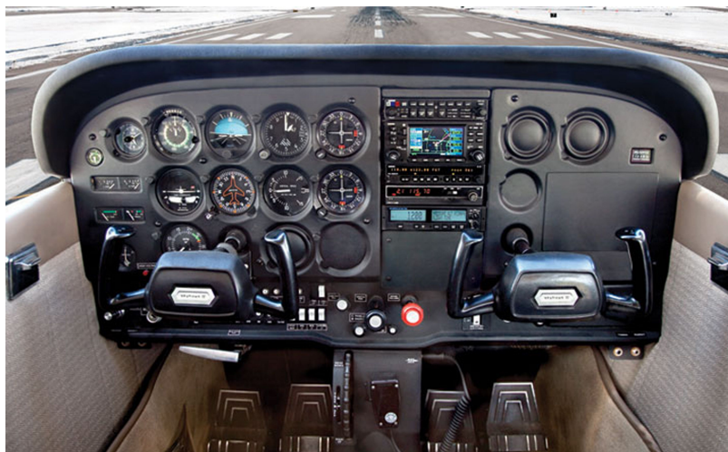
Figure 2.1: Single engine aircraft cockpit [47].
