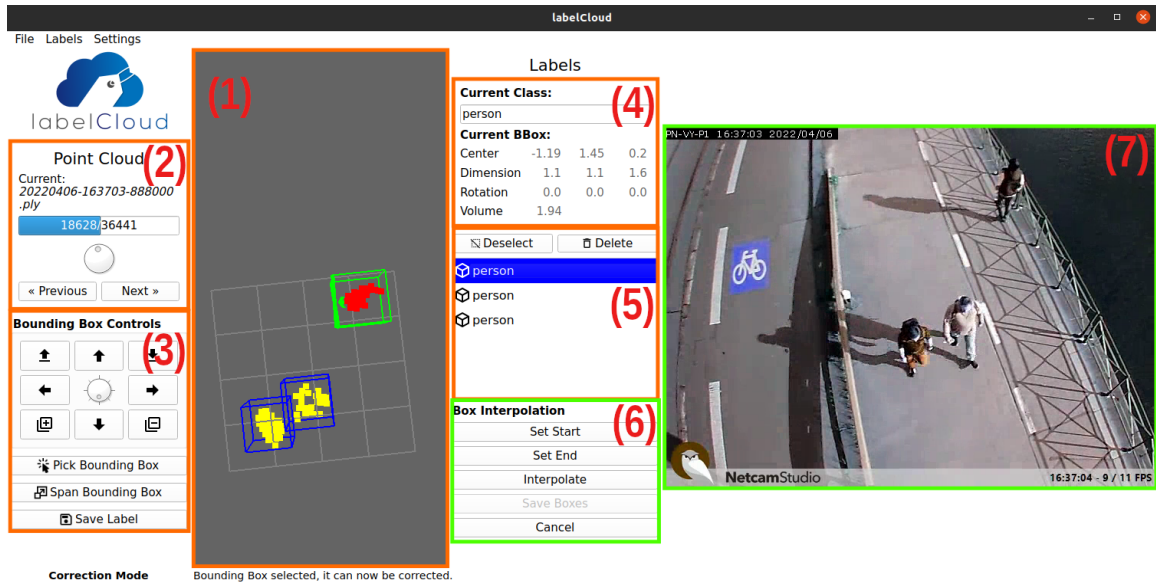
Figure 5.4: Extended labelCloud annotation tool. Green boxes show the contribution of this thesis to the GUI. (1) Point cloud visualization, (2) flow controls, (3) bounding box controls, (4) label information, (5) list of labels, (6) interpolation controls, (7) reference video frame.
