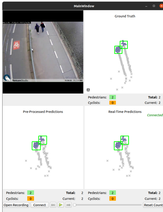
Figure 7.6: The visualizer application. From top left clock-wise: (1) referential video, (2) ground truth plot, (3) online predictions, (4) offline predictions.
