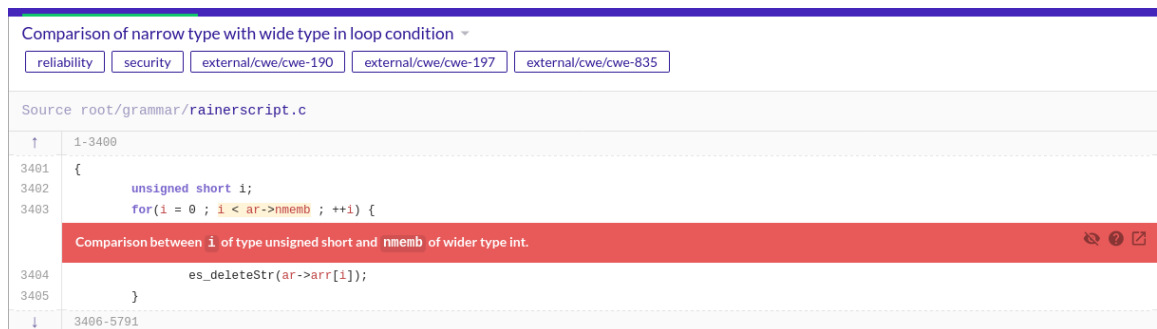
Figure 5.4: Example of a vulnerability detected by LGTM
