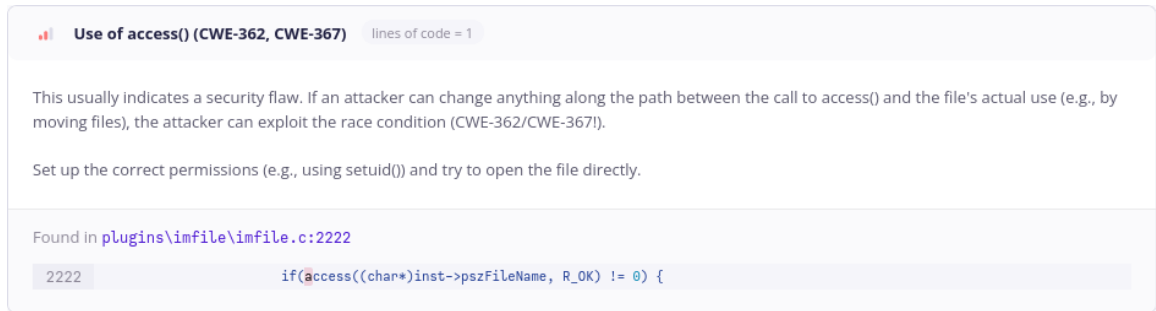
Figure 5.5: Example of a potential CWE detected by Codefactor
