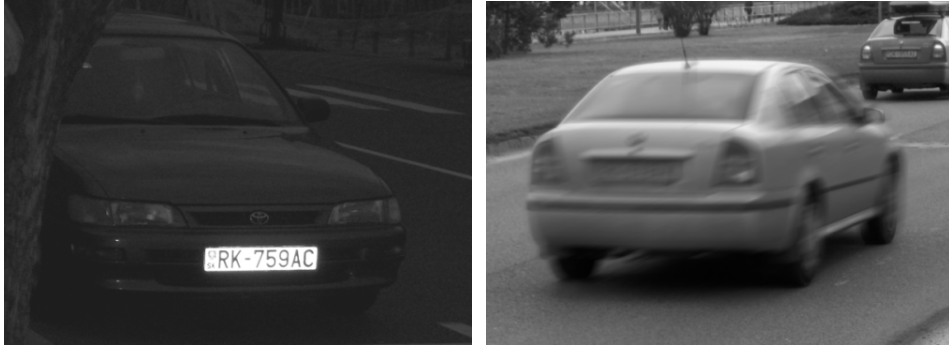
Figure 1.1: (a) Illumination makes detection of reflexive image plates easier. (b) Long camera shutter and a movement of the vehicle can cause an undesired motion blur effect.
