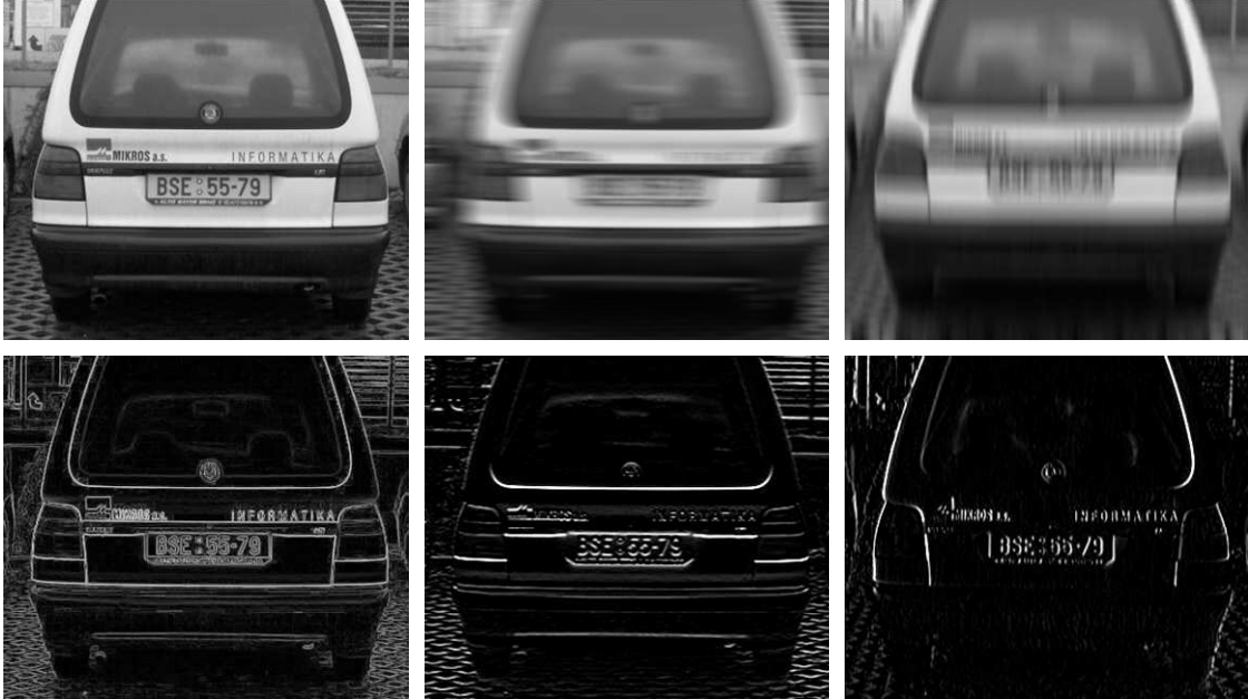
Figure 2.2: (a) Original image (b) Horizontal rank filter (c) Vertical rank filter (d) Sobel edge detection (e) Horizontal edge detection (f) Vertical edge detection
